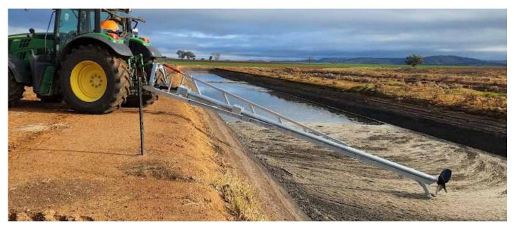
Storth Lagoon Mixers are built to last with the machine being fully galvanised and strengthened with a heavy duty box section placed underneath the mixer tube.
